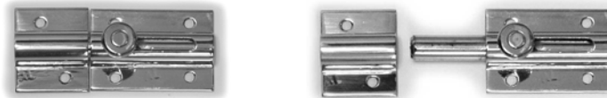
#92.080; small barrel bolt with strike plate; plate size: 50 x 36 mm 2" x 1 7/16"; strike: 30 x 36 mm; 1 3/16" x 1 7/16"; throw: 1 1/4". 304 stainless steel
